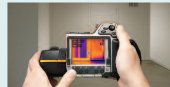
Infrared cameras quickly locate moisture related problems
