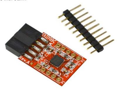
MOD-MPU9150 is 9-axis motion tracking device with 3-axis gyroscope, 3-axis accelerometer and 3-axis magnetometer in small 4x4 mm package.
