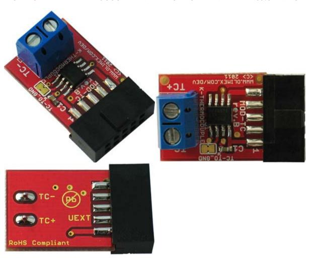
MOD-TC allow boards with <u>UEXT connector</u> to measure temperature with <u>TC-K-TYPE</u> K-type thermocouple. It have MAX6675 IC and allow temperature in range 0-1023.75C to be measured with 0.25C resolution.
