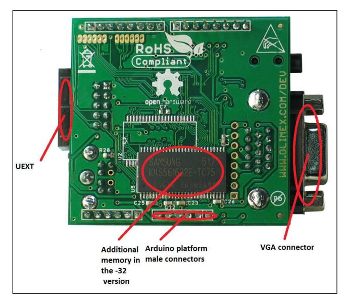
Note the base MOD-VGA version doesn't have the additional memory present on the picture of MOD-VGA-32.
