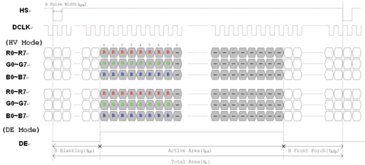
Figure 5: Horizontal Input Timing Diagram
