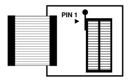
NOTE: Align PIN 1 of all devices with the arrows indicated.
