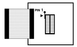
NOTE: Align PIN 1 of all devices with the arrows indicated.
