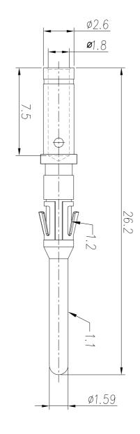
ECO-MATE, PIN CONTACT, MACHINE, 16-18AWG, SIZE 16
