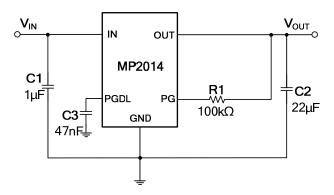
**Figure 5: Typical Application Circuit**
