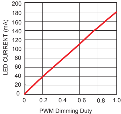
LED Current vs. PWM Dimming Duty
