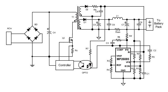
Figure 2— Adapter / Battery Charger Using MP26085 with Auxiliary Winding
