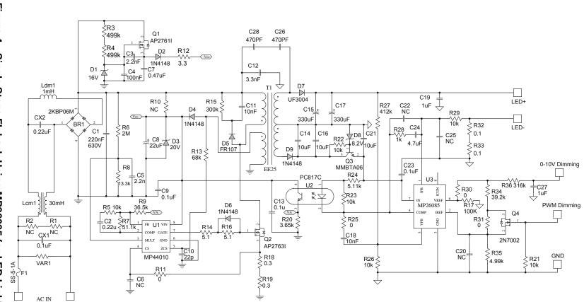
Figure 4– -Single Stage Flyback Using MP26085 for LED Lighting
