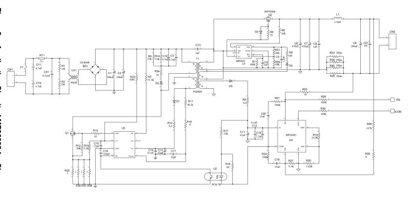
Figure 5— Application Circuit of MP26085 for Charger
