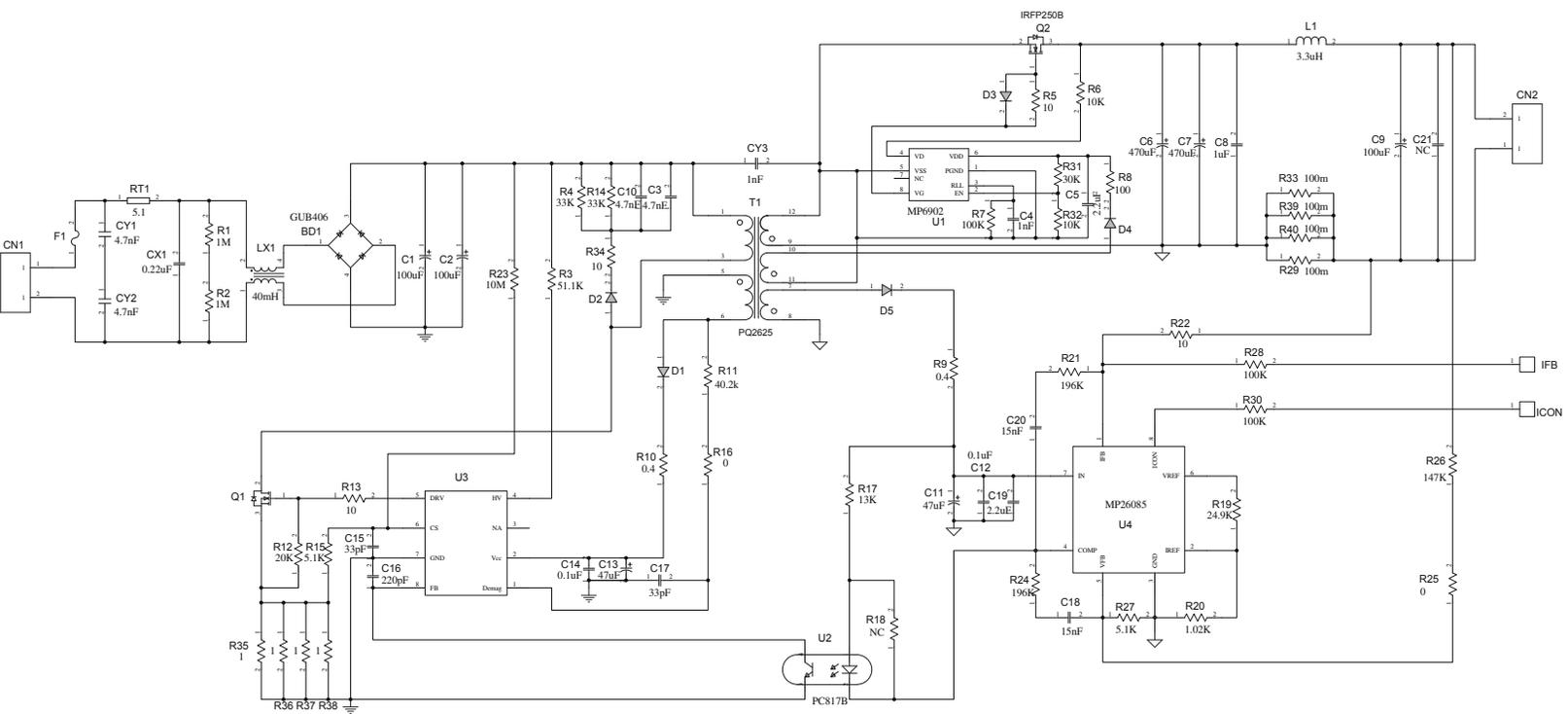
Figure 5— Application Circuit of MP26085 for Charger
