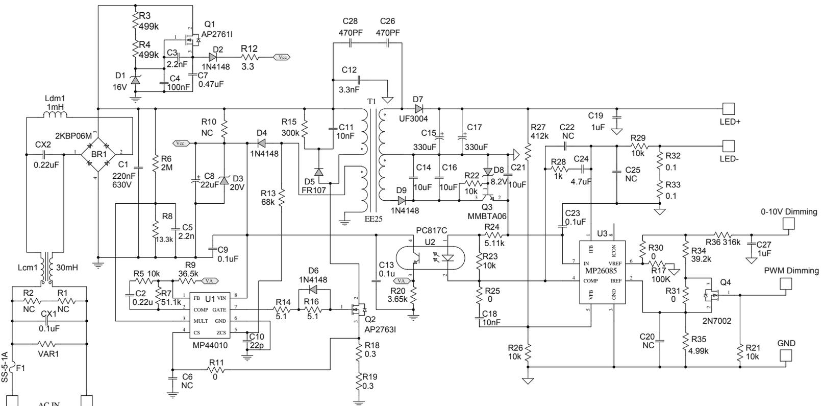
**Figure 4—Single Stage Flyback Using MP26085 for LED Lighting**
