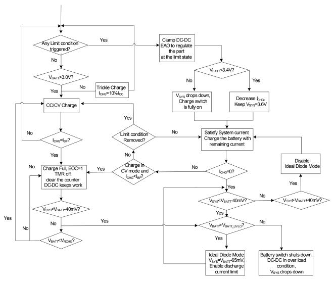
Figure 5— MP2625B Operation Flow Chart under No Fault Condition
