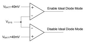
Figure 4— Ideal Diode Mode Enable/Disable
