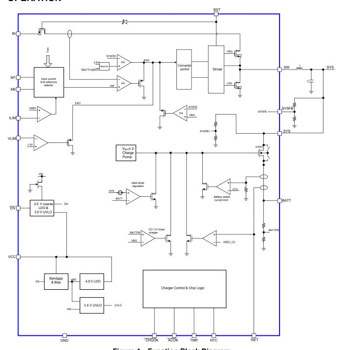
Figure 1—Function Block Diagram
