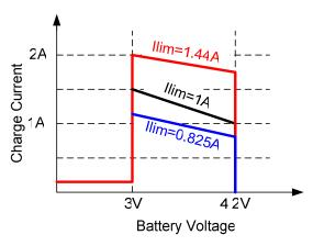
Figure 7—I<sub>CHG</sub> Variation with Different Input Current Limit
