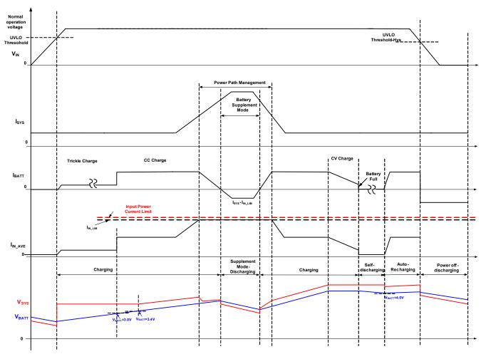
Figure 6— MP2625B Operation Process under No Fault Condition
