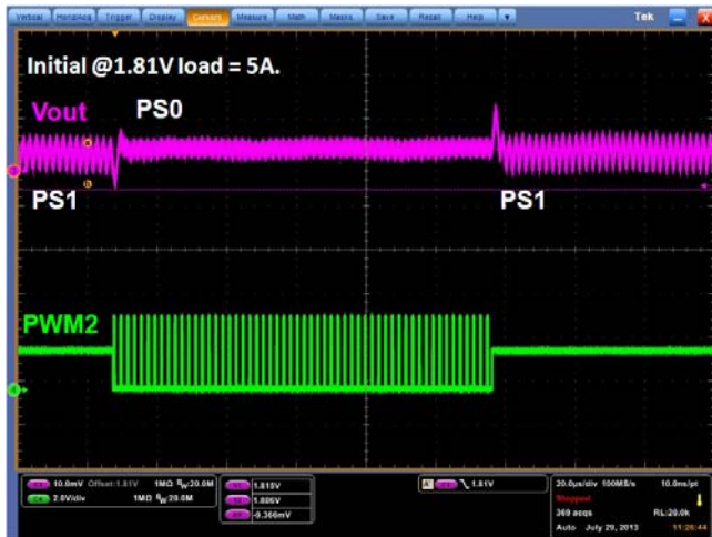
FIGURE 5(a). 1-Phase CCM →6-Phase →1-Phase CCM
