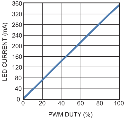
PWM Dimming Curve
