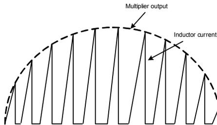
**Figure 4: Power-Factor Correction**
