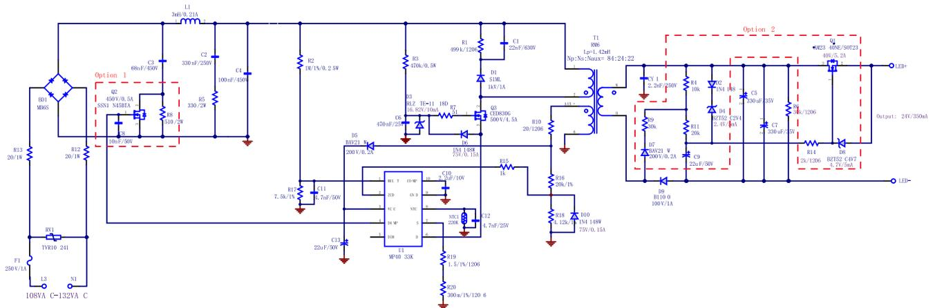
**Figure 21: A19 Bulb Driver, 120VAC/60Hz Input, Isolated Flyback Converter,  $V_O =24V$ ,  $I_O=350mA$
