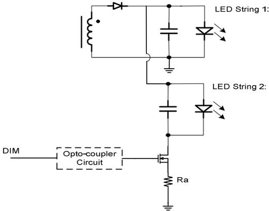
**Figure 16: Color Temperature and Brightness Control Circuit**
