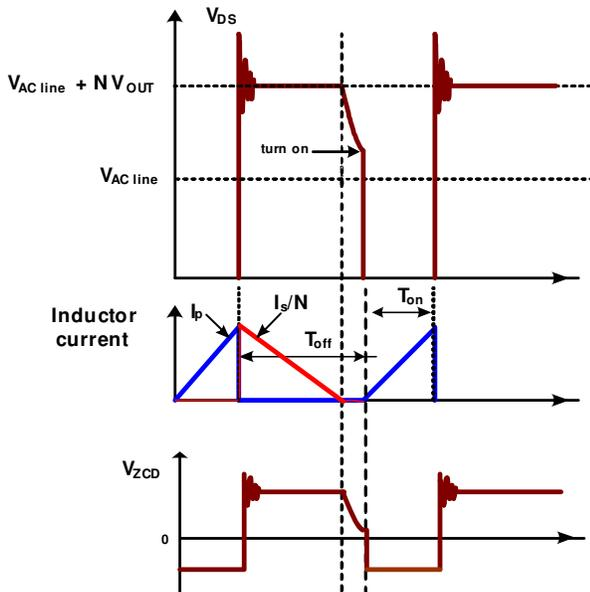
**Figure 2: Boundary-Conduction Mode**
