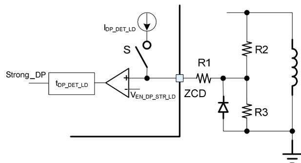
**Figure 15: Weak/Strong Dimming Pull Down Current Source Selection**
