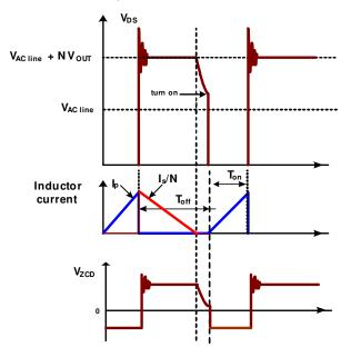
Figure 2: Boundary-Conduction Mode
