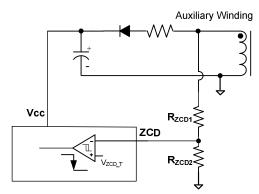
**Figure 3: Zero-Current Detector**
