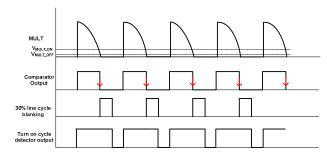
Figure 12: Dimming Turn-On Cycle Detector
