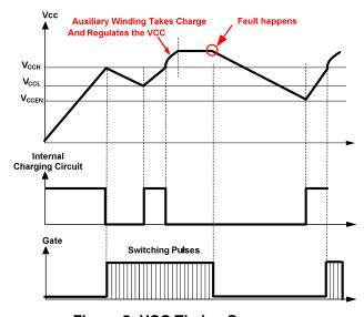
Figure 5: VCC Timing Sequence
