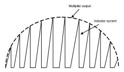
Figure 4: Power-Factor Correction
