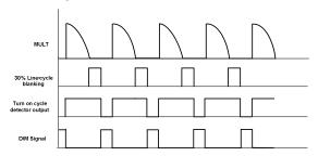
Figure 17: Dim Signal Logic
