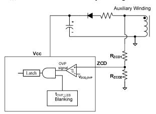
Figure 7: OVP Sampling Circuit
