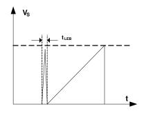
Figure 6: Leading-Edge Blanking
