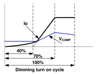
Figure 14: Trailing Edge Dimming Curve
