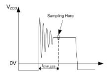
Figure 8: ZCD Voltage and OVP Sampling
