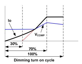
Figure 13: Leading Edge Dimming Curve
