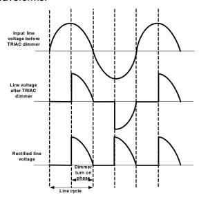
Figure 10: Leading Edge Dimmer Waveforms
