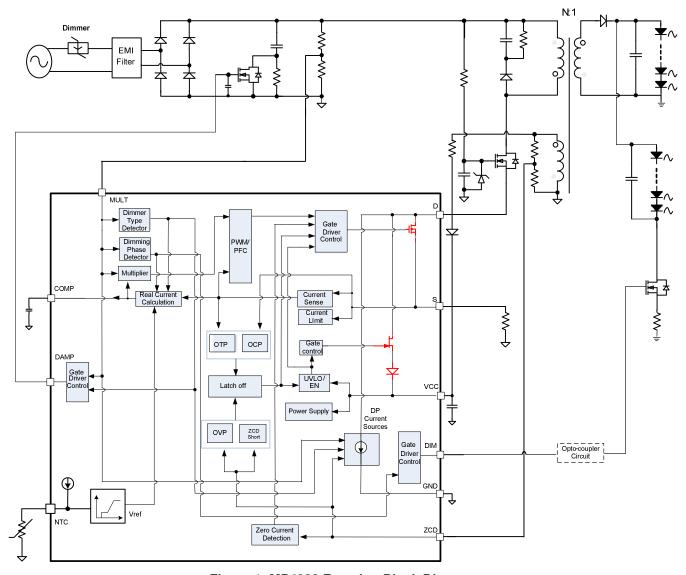
Figure 1: MP4033 Function Block Diagram
