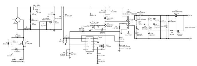
Figure 20: A19 Bulb Driver, 230VAC/50Hz Input, Isolated Flyback Converter,  $V_0$  =24V,  $I_0$ =420mA EVB Model: EV4033-K-00A
