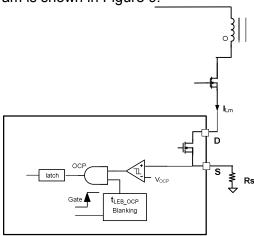
**Figure 9: Over-Current Protection Circuit**
