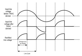
Figure 11: Trailing Edge Dimmer Waveforms
