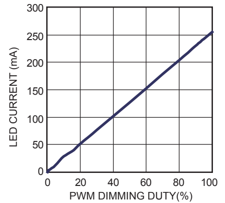
PWM Dimming Linearity @ 200Hz
