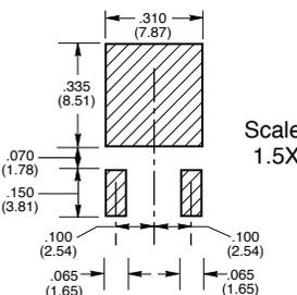
**Soldering Note:** During surface mount soldering the soldering temperature profile must not cause the metal tab of this device to exceed 220°C.
