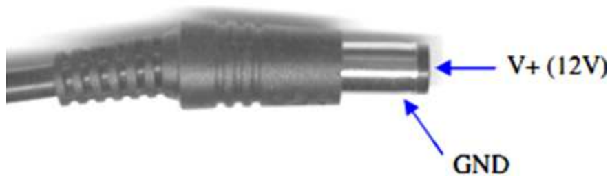
Figure 2. 2.1 mm Power Connector
