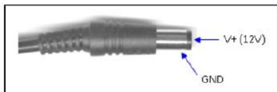
Figure 3: 2.1 mm Power Connector
