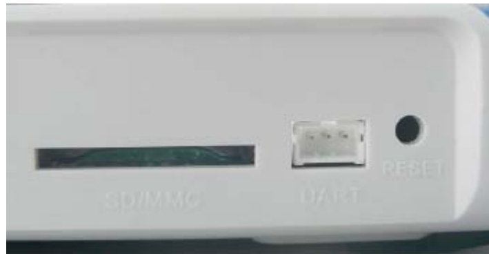
Figure 4. UART Port and SD/MMC Slot on MPC8308-NSG
