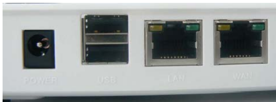
Figure 3. Ethernet and USB Ports on MPC8308-NSG
