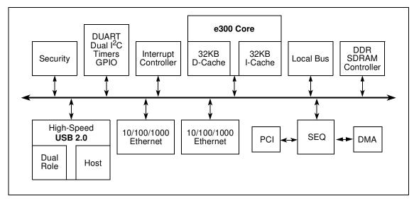
Figure 1. MPC8347E Block Diagram
