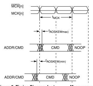
Figure 5. Timing Diagram for  $t_{\text{AOSKEW}}$  Measurement
