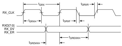
Figure 9. GMII Receive AC Timing Diagram
