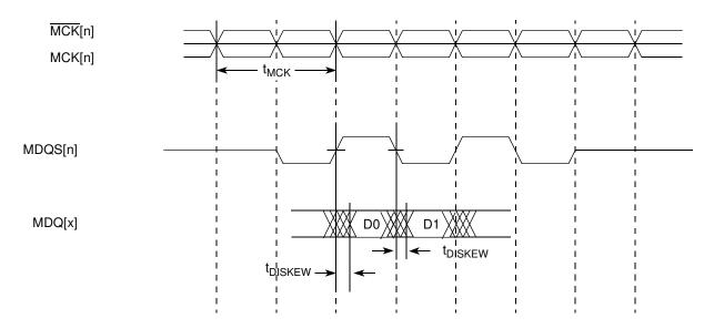
Figure 4. DDR Input Timing Diagram
