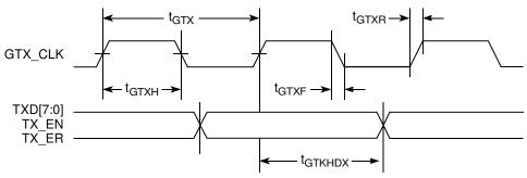
Figure 8. GMII Transmit AC Timing Diagram
