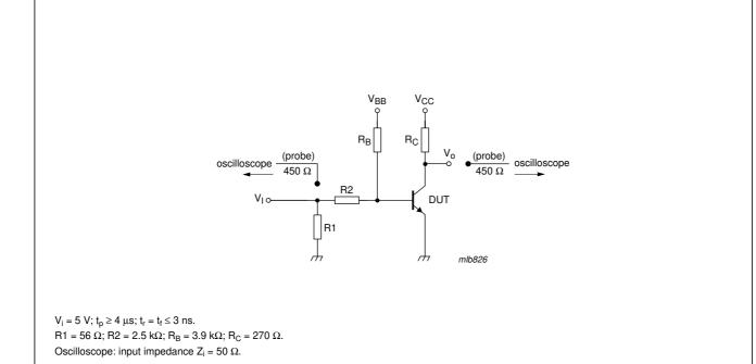
Fig.2 Test circuit for switching times.
