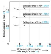
These curves show the characteristics with the maximum sensing range set to 40 mm 1.575 in, 30 mm 1.181 in and 20 mm 0.787 in, with white non-glossy paper (10 × 10 mm 0.394 × 0.394 in).
