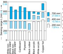
These bars indicate the sensing range with the respective objects when the distance adjuster is set to a sensing range of 700 mm 27.559 in, 400 mm 15.748 in and 200 mm 7.874 in long, respectively, with white non-glossy paper.
