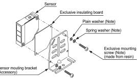
Note: Attached with the exclusive insulating board.
