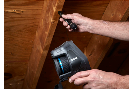
Use MR40 to confirm whether the cold spot found in a thermal image is moisture
