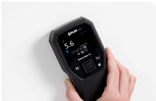
Verify moisture with pinless measurements
