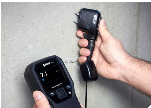
External pin probe for resistive moisture readings
