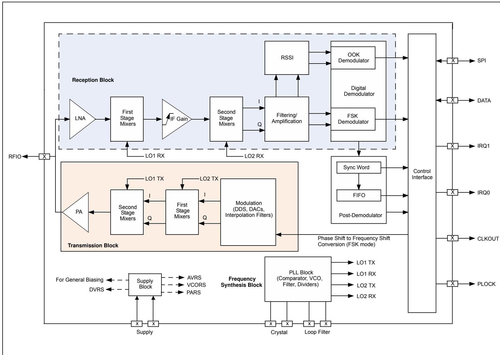
**FIGURE 1-2: MRF89XA TO MICROCONTROLLER INTERFACE (NODE) BLOCK DIAGRAM**
