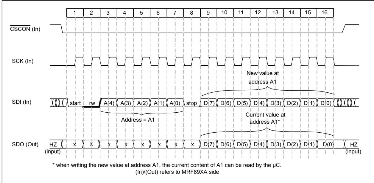
**Read Register** - To read the value of a Configuration register, the timing diagram illustrated in Figure 2-13 should be followed by the host microcontroller.
