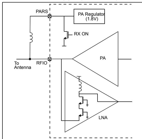
The PA and the LNA front-ends in the MRF89XA, which share the same Input/Output pin, are internally matched to approximately 50 $\Omega$ .
