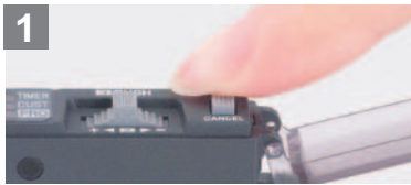
MODE Pressing the switch selects or cancels the operating mode
