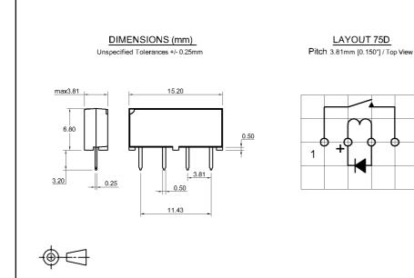
Coil Data at 20 ℃ Conditions Тур Min Max Unit Coil resistance 450 500 550 Ohm Coil voltage 5 VDC Rated power 50 mW Pull-In voltage 3.75 VDC Drop-Out voltage VDC 0.75
