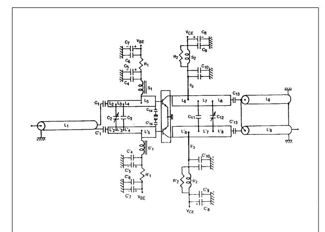
C1, C1, C1, C3, C3 :  $50\Omega$  Printed Transmission Line Length 3mm L4, L3 :  $50\Omega$  Printed Transmission Line Length 9.5mm C2 : 4.5pF Adjustable Johanson L5, L5 :  $39\Omega$  Printed Transmission Line Length 7mm C3 : 4.7pF, ATC 100A L6, L6 :  $39\Omega$  Printed Transmission Line Length 15mm C4, C4, C6, C9, C9, C9, L7, L7 :  $39\Omega$  Printed Transmission Line Length 8mm
