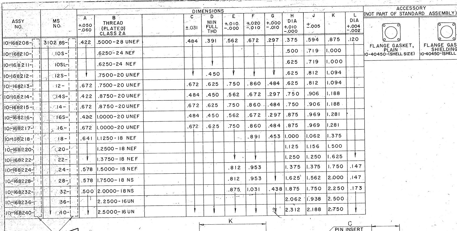
8 ALL 10-8 61-ASSEMBLIES TO BE ASSEMBLED PER 9-3103-1 & TESTED PER 9-3106-5 SUCH UNITS MEET THE REQUIREMENTS OF MS3102A PER MIL-C-5015D. INSERTS & CONTACTS ARE REMOVABLE
