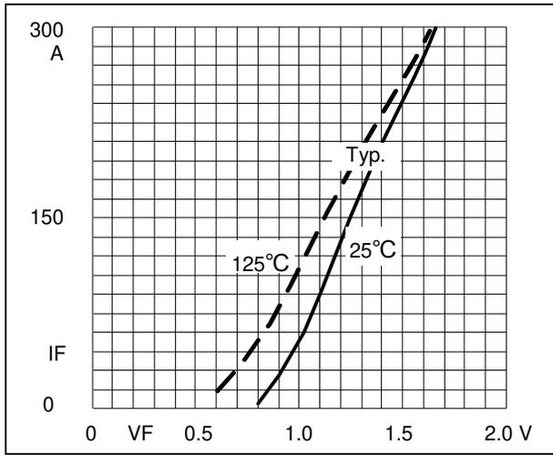
**Fig1. Forward Characteristics**
