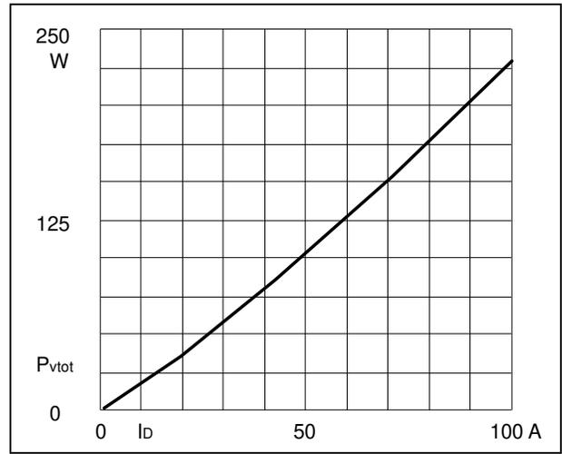
**Fig2. Power dissipation**
