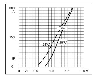
Fig1. Forward Characteristics
