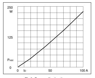
Fig2. Power dissipation
