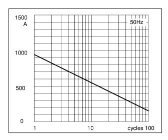
Fig4. Max Non-Repetitive Forward Surge Current
