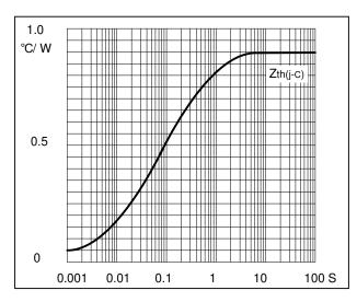
Fig3. Transient thermal impedance
