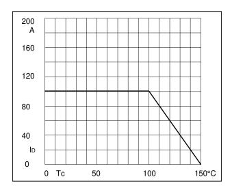
**Fig5.Forward Current Derating Curve**
