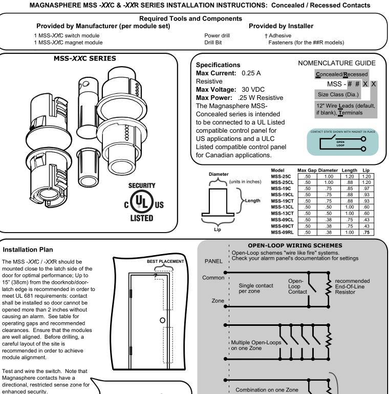
Insert the switch module into the hole of the frame. Insert the magnet module into the hole in the door. †Adhesive (such as RTV) is recommended to assure a secure fit. Adhesive may be necessary for materials which are too thick for retaining barb deployment (wood or thick metal). Check the operation of the installed switch. -XXR models are provided with a wide flange and pilot holes for (optional) fasteners..
