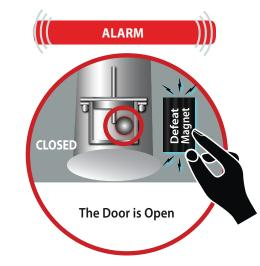
MAGNASPHERE's contact is a spherical magnet and operates in a defined activation zone directed toward the door magnet.
