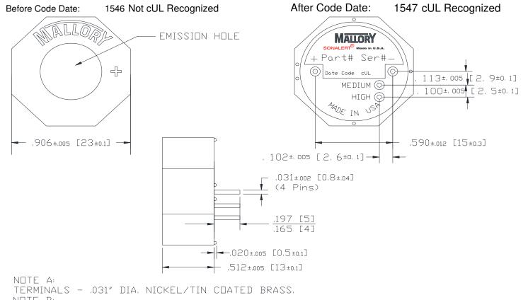
MOUNTING- INSERT INTO PRINTED CIRCUIT BOARD AND HAND OR MACHINE SOLDER, UNITS ARE SUITABLE FOR WAVE SOLDERING. BOARDS ARE NOT SUITABLE FOR WASH. RECOMMENDED MAXIMUM TEMPERATURE AND TIME DURATION FOR WAVE SOLDERING IS +270°C AND 3 SECONDS RESPECTIVELY.
