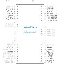
Universal Socket Connectivity. Multi-Tech's universal socket is a flexible, comm-port architecture that provides cellular, Ethernet, PSTN or Wi-Fi network access with interchangeable communications devices. This means you can utilize one system design and populate it with your connectivity device of choice accommodating multiple connectivity requirements. In addition, you are assured a seamless migration to future technologies.
