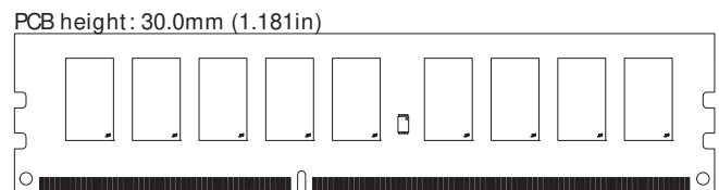
Figure 1: 240-Pin UDIMM (MO-269 R/C E)
