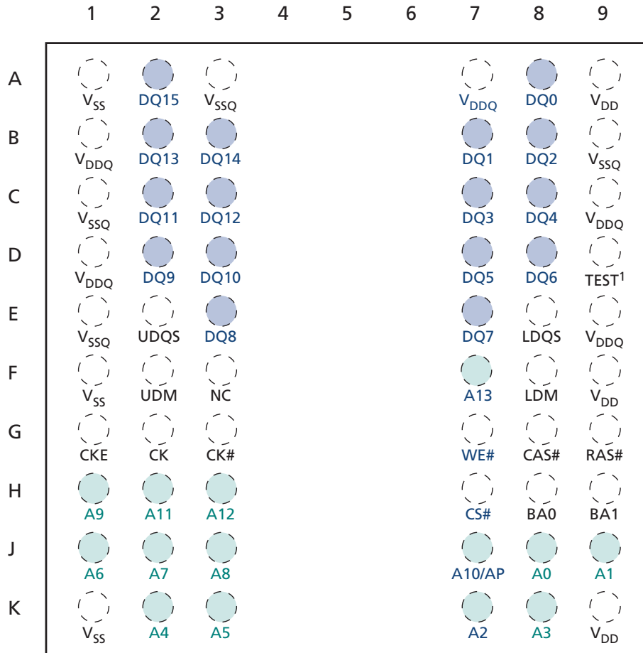
Figure 4: 60-Ball VFBGA – Top View, x16 only
