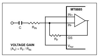
Figure 3 - Single-Ended Input Configuration
