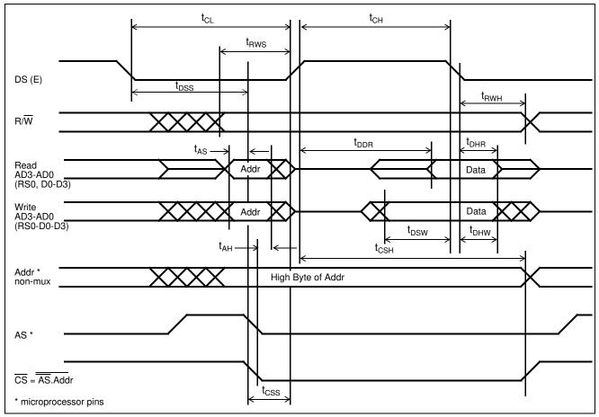
Figure 16 - Motorola BUS Timing Diagram
