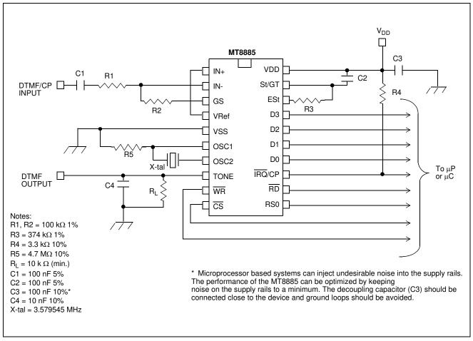
Figure 13 - Application Circuit (Single-Ended Input)
