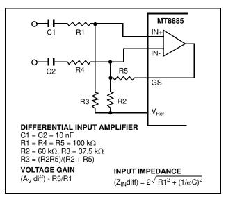
Figure 4 - Differential Input Configuration
