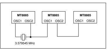
Figure 11 - Common Crystal Connection
