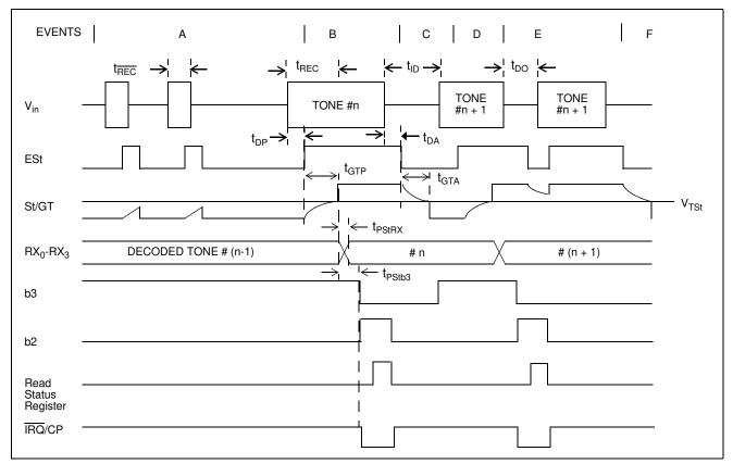
Figure 7 - Receiver Timing Diagram
