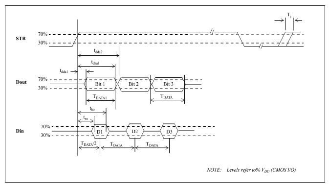
Figure 6 - SSI Asynchronous Timing Diagram
