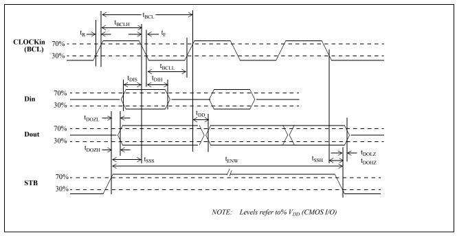
Figure 5 - SSI Synchronous Timing Diagram
