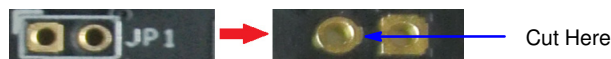
Figure 7. Top and Bottom View of Shorted Jumper. The Bottom View Shows the Trace Location to Cut for Current Measurement
