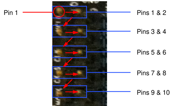
Figure 6. Pin Locations and Assignments of Grouped Jumpers. Pin 1 is Located at the Top-Left Corner and Increases in a Zigzag Fashion Shown in the Picture (P11 and P15 has different orientation)
