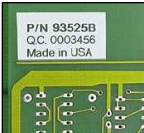
Circuit board labeling
