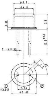
1- cathode, 2 -anode, all dimensions in mm, tolerance: ±0.2
