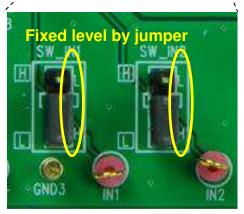
Jumper indicated on the left is adopted on this evaluation board to set operation of the TB6642FTG. To select the function by the jumper, supply the voltage of high level by VDD pin.
