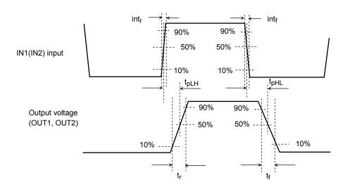
Note: When the signal is input to IN1 (IN2) pin, we recommend that intr, intf are provided more than 10ns in order to avoid malfunction in the input switching noise. For example, please connect the capacitor between IN1 (IN2) pin and GND.
