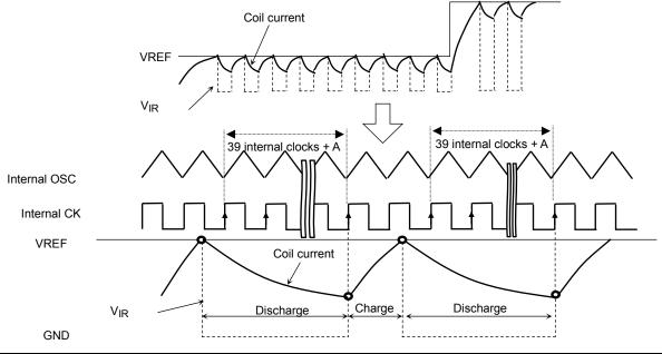
(4) Operation on change of predetermined current value (when in Discharge mode) The TB67H301FTG enters Discharge mode as VIR reaches the predetermined voltage (VREF) and then transits to Charge mode after 39 internal clocks + A. However, if VIR > VREF at the time, the TB67H301FTG goes back to Discharge mode. If VIR < VREF after another 39 internal clocks + A, then the TB67H301FTG enters Charge mode and stays until VIR reaches VREF.
