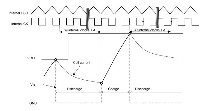
Due to the peak current detection technique, the average current value of the constant-current operation shall be smaller than the predetermined value. Because this depends on characteristics of used motor coils, precise identification of the used motor coils must be performed when determining the current value.
