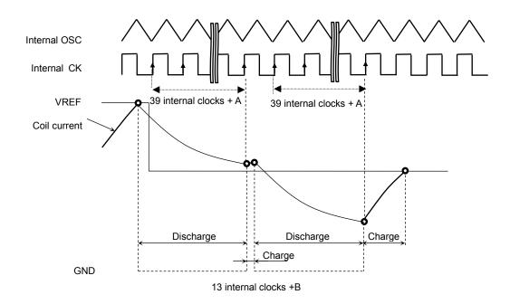
(5) Operation on change of predetermined current value (when in Charge mode) Even though VREF reaches the predetermined current value, Discharge mode continues for 39 internal clocks + A after that. And then Charge mode is entered.
