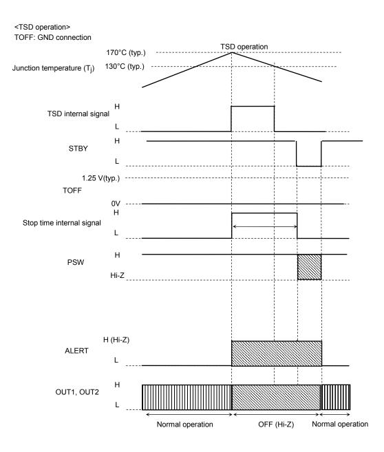
Note: The TSD circuit is activated if the absolute maximum junction temperature rating (T<sub>j</sub>) of 150°C is violated. Note that the circuit is provided as an auxiliary only and does not necessarily provide the IC with a perfect protection from any kind of damages.
