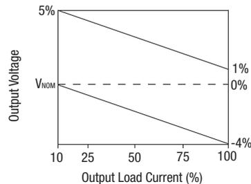
The voltage tolerance envelope shows typical load regulation characteristics for this product series. The tolerance envelope is the maximum output voltage variation due to changes in output loading and set point accuracy.
