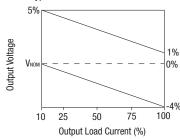
The voltage tolerance envelope shows typical load regulation characteristics for this product series. The tolerance envelope is the maximum output voltage variation due to changes in output loading and set point accuracy.
