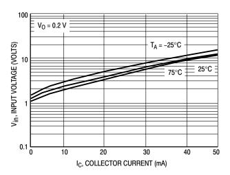
Figure 16. Input Voltage versus Output Current
