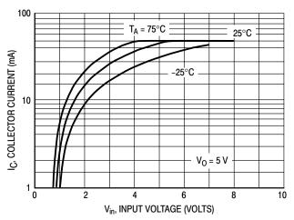
Figure 40. Output Current versus Input Voltage
