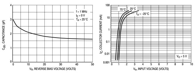
Figure 19. Output Capacitance
