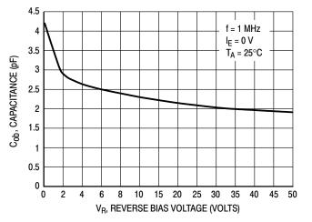
Figure 39. Output Capacitance
