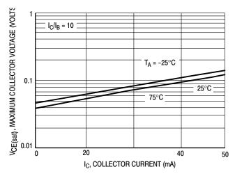
Figure 7.  $V_{CE(sat)}$  versus  $I_C$
