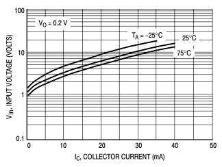
Figure 26. Input Voltage versus Output Current
