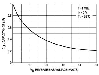
Figure 29. Output Capacitance
