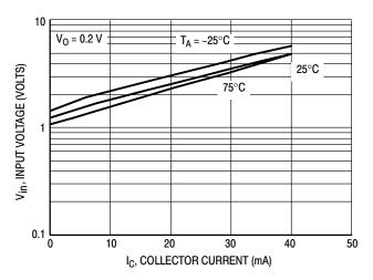
Figure 6. Input Voltage versus Output Current
