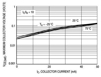
Figure 12. V<sub>CE(sat)</sub> versus I<sub>C</sub>
