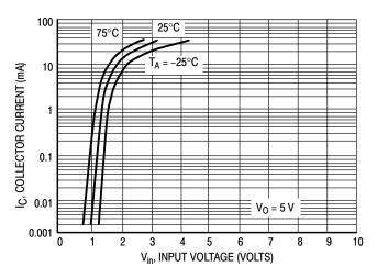
Figure 10. Output Current versus Input Voltage
