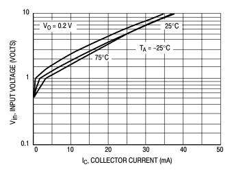
Figure 41. Input Voltage versus Output Current
