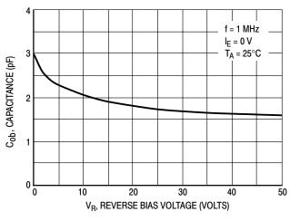
Figure 9. Output Capacitance
