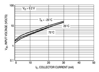
Figure 21. Input Voltage versus Output Current
