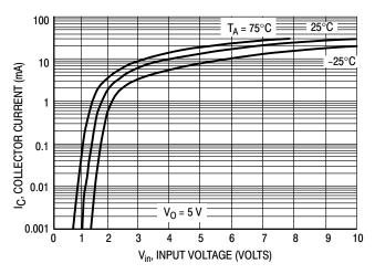
Figure 30. Output Current versus Input Voltage
