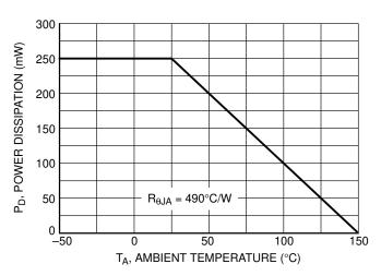
Figure 1. Derating Curve
