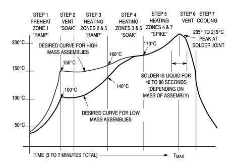
Figure 46. Typical Solder Heating Profile
