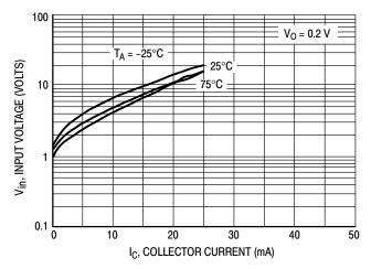
Figure 31. Input Voltage versus Output Current
