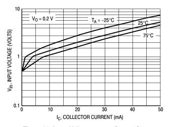
Figure 36. Input Voltage versus Output Current
