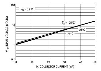
Figure 11. Input Voltage versus Output Current
